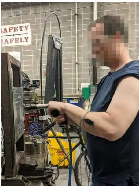
Figure 8. Riveting with support
